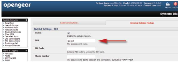
**Note:** Your GSM carrier may have provided you with connection details. However, you generally will only need to enter your provider's APN and leave the other fields blank. If provided a Pin Code you may need to use it to unlock the SIM card.
