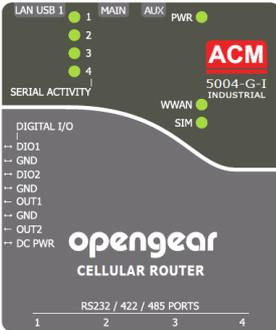
The **ACM5004- I** has a dedicated I/O (*DIO1* & *DIO2*) and output only pins (*OUT1* & *OUT2*), the later having inverting outputs with higher voltage/current transistors. These four digital I/O ports present on a green connector block:
