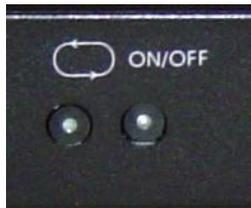
Cycle (left): Select power outlet to manually control
