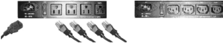
For the European/Australian model (IEC320-C13 220-250V outlets) the individual max output current per outlet is 6A and the total max output current for the 4 outlets is 10A. Use a power IN cable with 10A current rating and use power OUT cable with 10A rating for each power outlet
