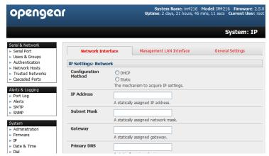
The second Ethernet network port (*ETH2*) is inactive by default. It can be set up for failover/OoB access (refer User Manual) or as a management gateway/LAN:
