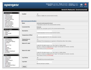
Then configure the attached sensors as alarms using the **Serial & Network: Environmental** menu
