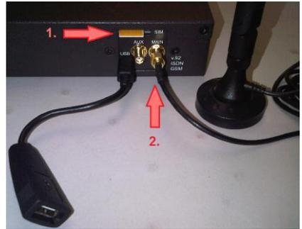
Complete to Step 4 (*Configure Serial and Network Devices*) in the QSG then connect to your wireless carrier as detailed below.
